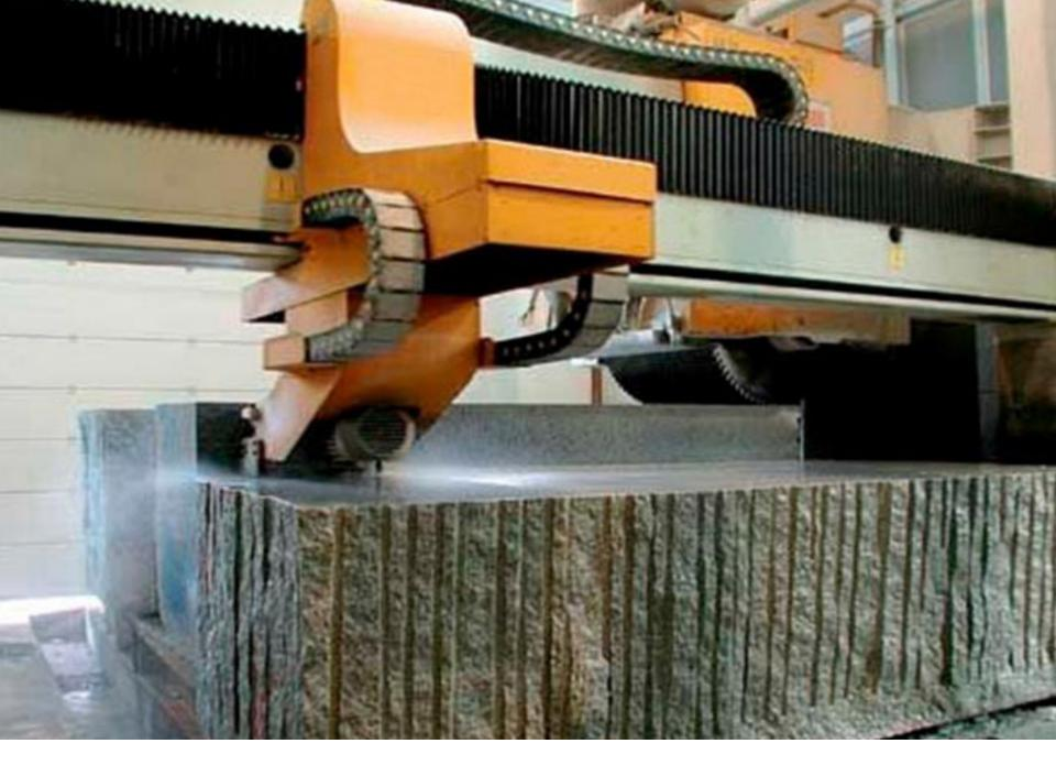
Rough edges & blemishes being carefully trimmed away to even out the surface of the block.
