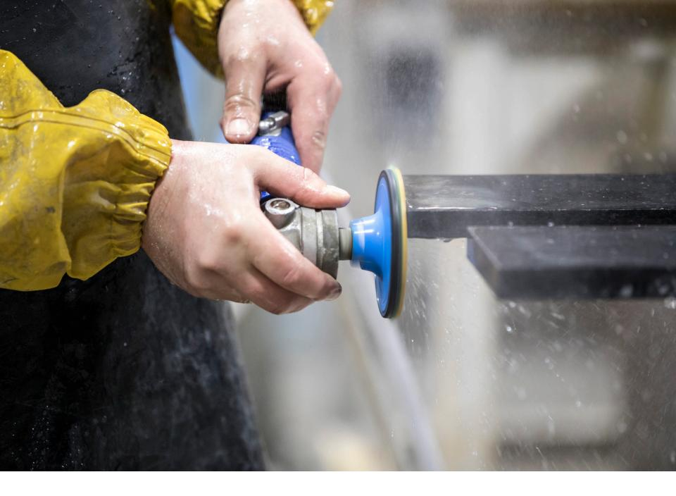
Polishing the stone to remove the excess epoxy resin to acquire mirror-like perfection.
