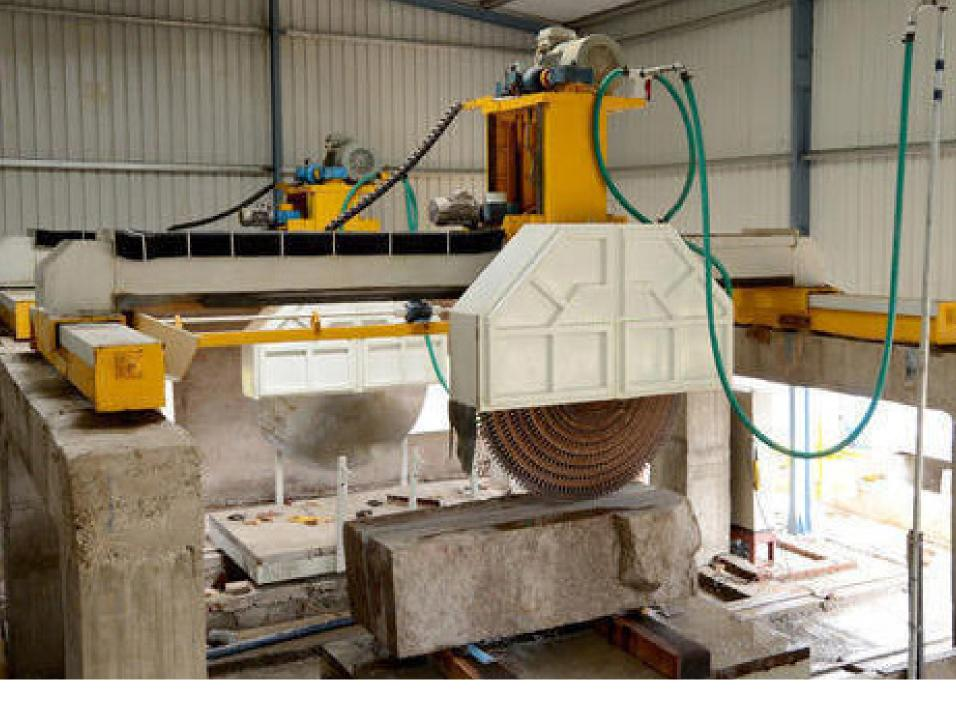
Thickness Calibration; once the block has been shaped, it is then cut.
